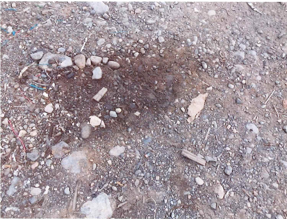
Photo 12: Example of the soil surface staining from small spills at 240 Okotoks Road.
