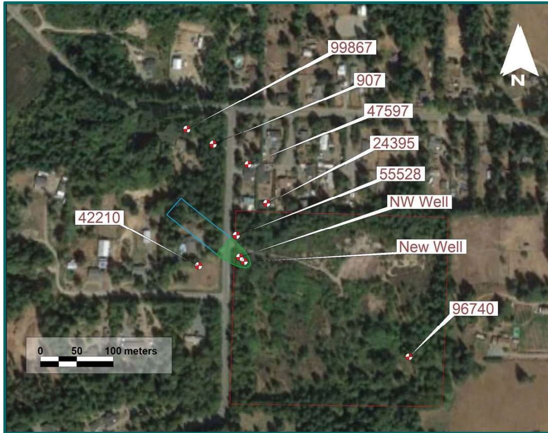
Figure 6. Illustration of predicted water well capture zones: 100 days (green) and 1-year (blue) times-of-travel. Local water wells are indicated by their well tag numbers.
