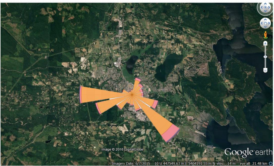
Duncan Cairnsmore PM2.5 Pollution Rose – Summer months (Jun, Jul, Aug) for all years (2010-2015 data).
