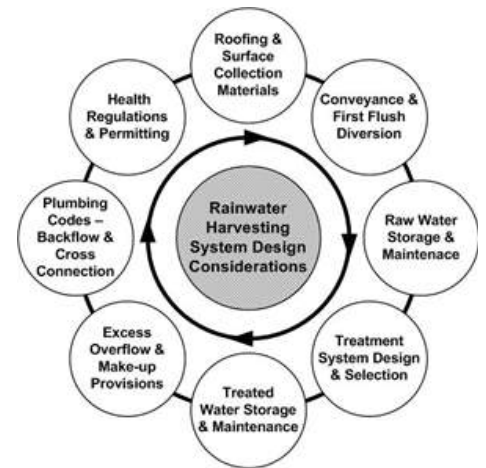
Key Eight Rainwater Harvesting System Design Considerations (Exall, K., and T.D. Vassos, 2012)
