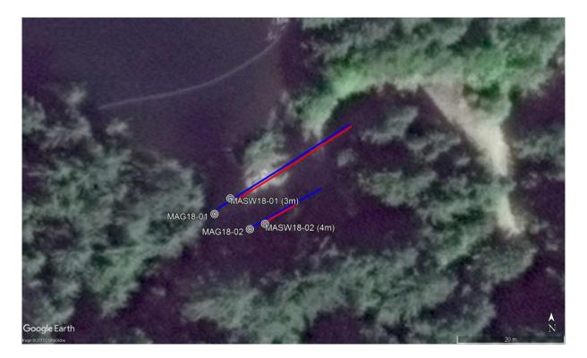
Google Earth image indicating the locations of MASW profiles (red) and Magnetometer profiles (blue). The numbers in brackets represent where the first data begin with respect to the start of the cross-section.
