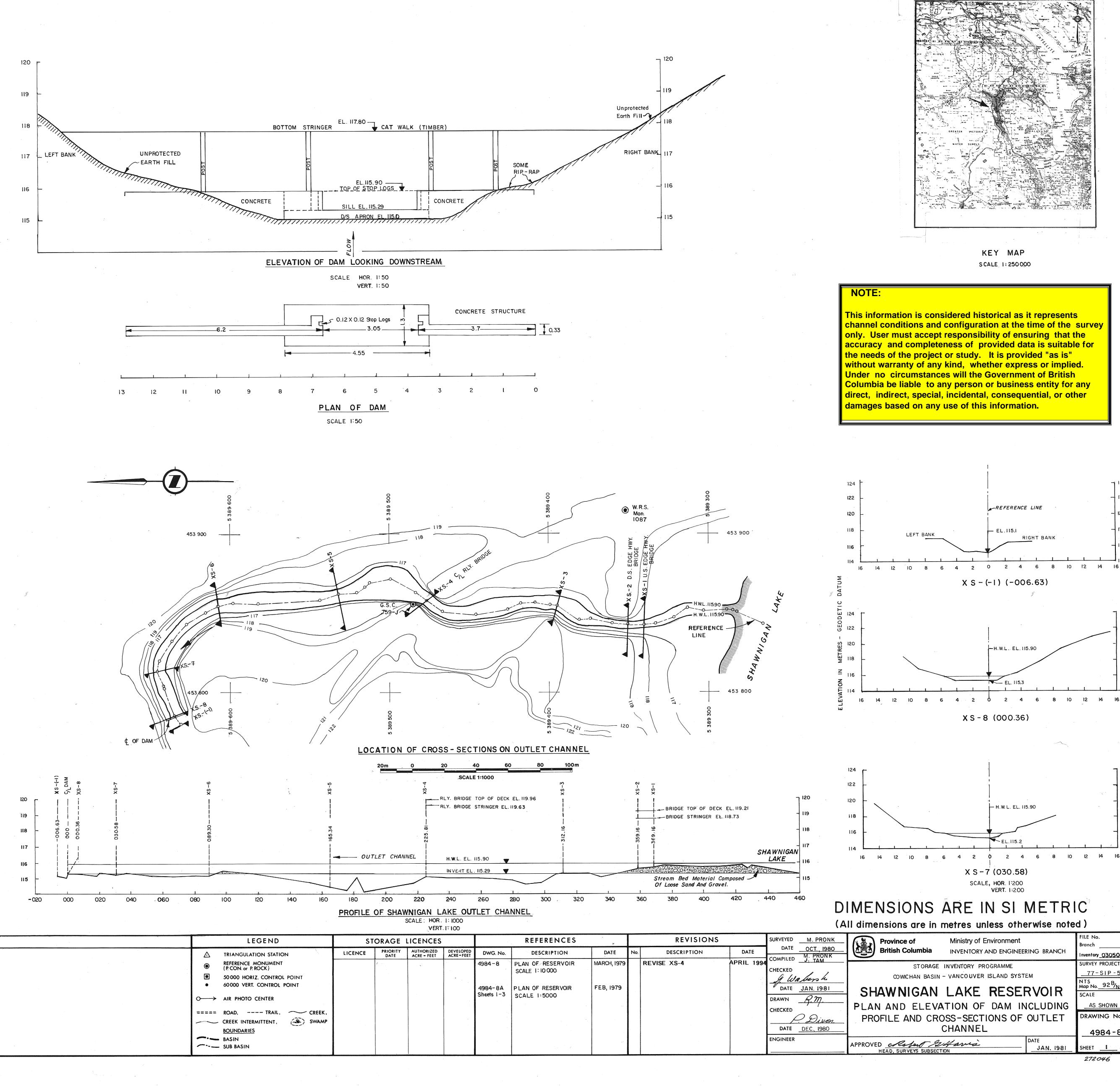
KEY MAP SCALE 1:250000 REFERENCE LINE - EL.115.1 RIGHT BANK X S - (-1) (-006.63) -H.W.L. EL. 115.90 XS-8 (000.36) H.W.L. EL. 115.90 Q 2 4 6 8 10 12 14 16 X S - 7 (030.58) SCALE, HOR. 1200 VERT. 1200 FILE No. Branch INVENTORY AND ENGINEERING BRANCH Inventory\_0305080-36 SURVEY PROJECT No. 77-SIP-5 NTS Map No. 92<sup>B</sup>/NW SCALE AS SHOWN DRAWING No. 4984-8B DATE JAN. 1981 SHEET \_\_\_\_\_ of 272046 DD
