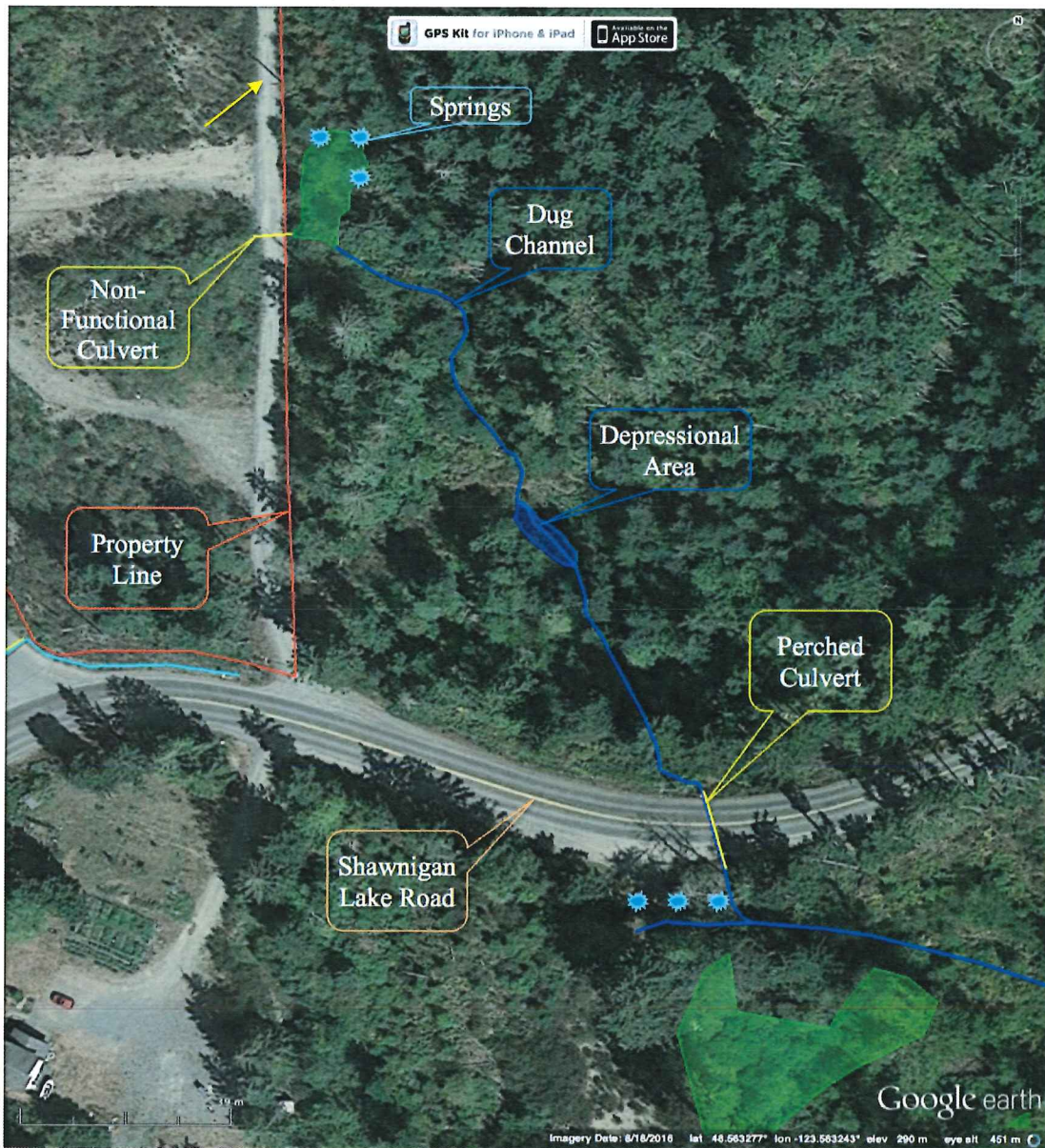
Figure 6: Sketch map of the unnamed tributary stream that flows into Saanich Inlet showing culvert and spring locations. Note this image is intended for illustrative purposes only and all notations are approximate. A B.C. Hydro power line lies along the eastern property line; shadows of the power poles can be seen on the gravel driveway (yellow arrow).
