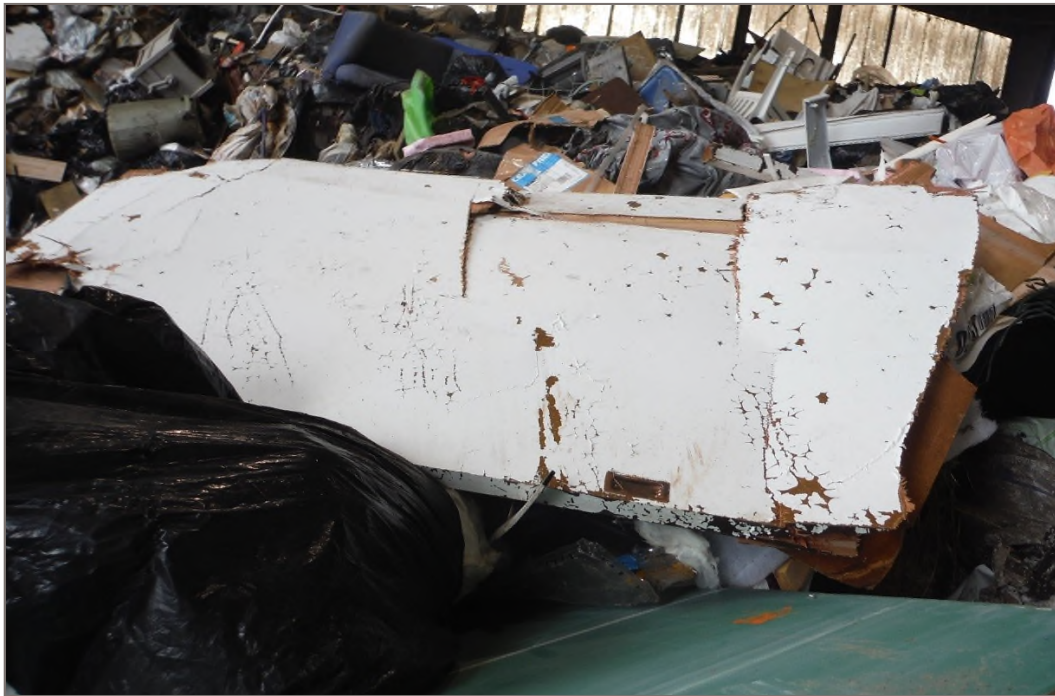
Photo 11: C&D – Large piece of contaminated wood, black bags, durable plastics, and bulky objects identified.
