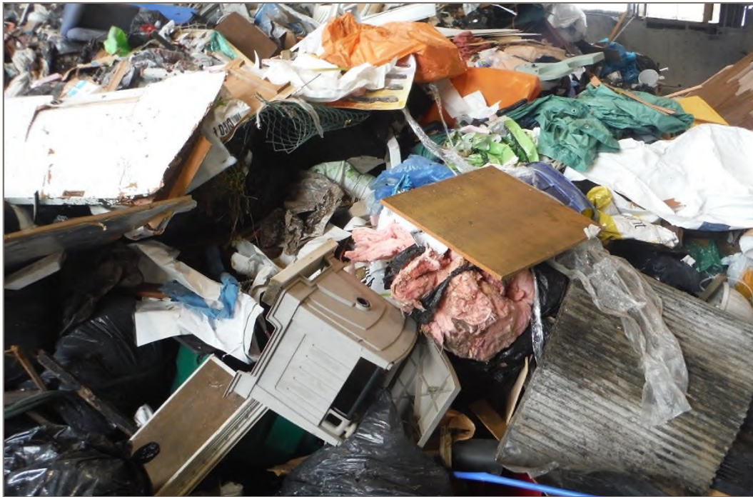
Photo 9: C&D – Contaminated wood, clean wood, durable plastics, metals, other building material (insulation) among others identified.
