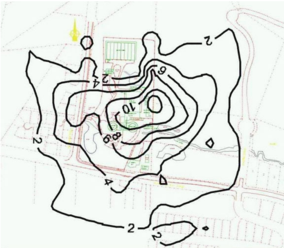
The Results of an Odour Model Showing Isoleths of Dilutions to Threshold Numbers
