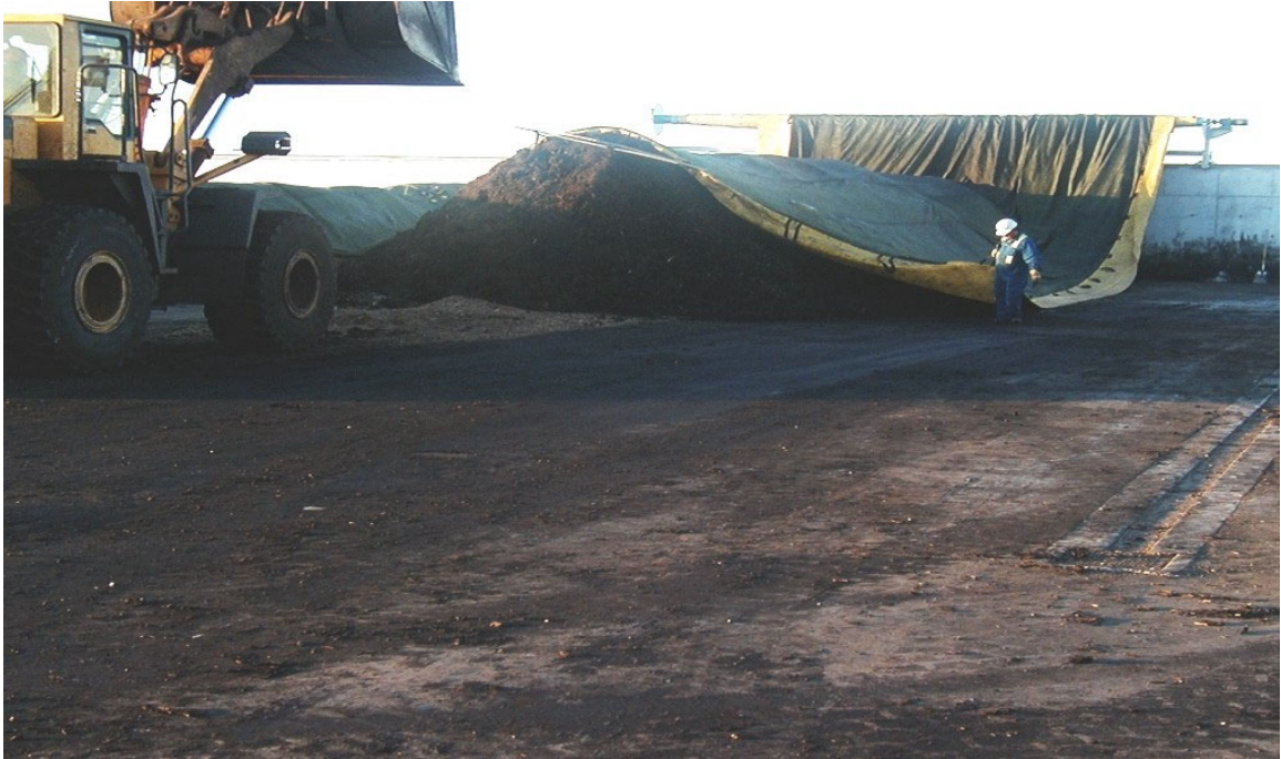
An Aerated Static Pile System with a Fabric Cover (Gore™) for Moisture and Odour Control
