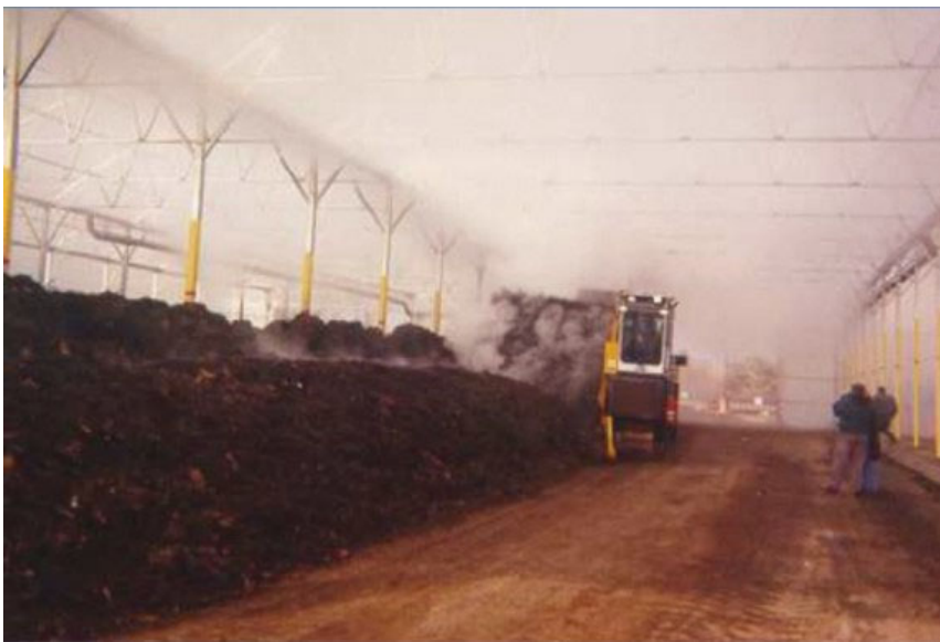
Windrow Composting Inside a Building (showing a self-propelled elevating turner)
