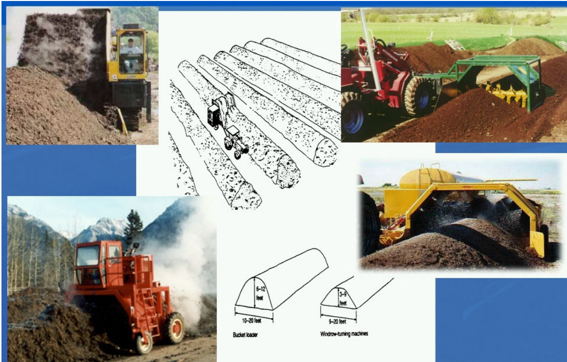
Windrow Composting Schematic and Example Windrow Turners
