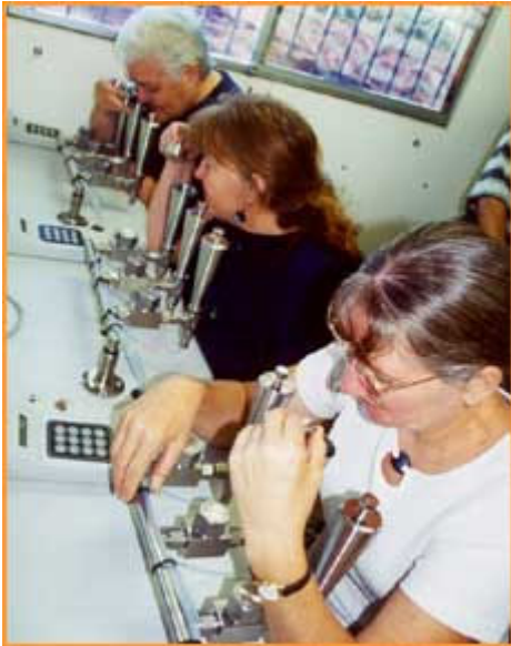
An Odour Panel testing an odour with a dynamic Olfactometer
