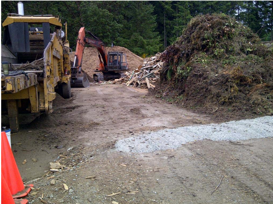
Photo 6: Piles of wood and garden waste in the chipping area. Area has a concrete floor and the storm water is collected.
