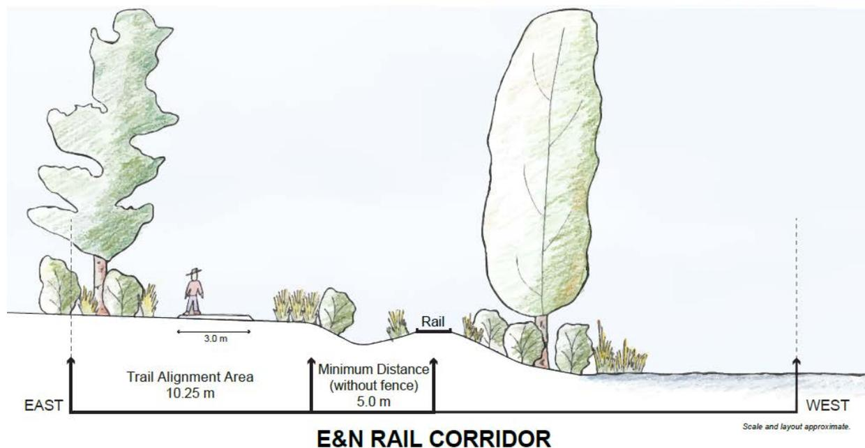
**Figure 5.4: Example of Rail with Trail Cross Section**
