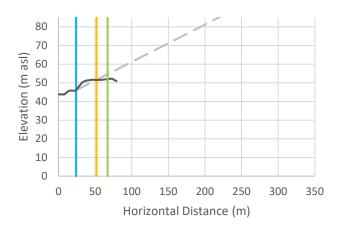
Cross-Section r-13: Vertical exaggeration = 2.5. The black line is the crosssectional data. The blue line is the toe of slope, the orange line is the calculated setback, and the green line is the calculated setback plus 15 m.
