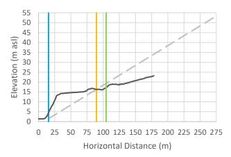
Cross-Section 29: Vertical exaggeration = 3. The black line is the cross-sectional data. The blue line is the Natural Boundary position with 1 m SLR, the orange line is the calculated setback, and the green line is the calculated setback plus 15 m.
