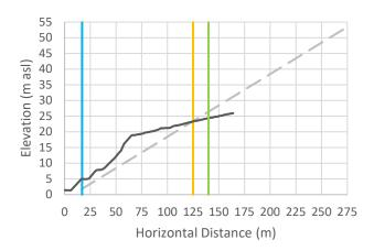
Cross-Section 45: Vertical exaggeration = 3. The black line is the cross-sectional data. The blue line is the Natural Boundary position with 1 m SLR, the orange line is the calculated setback, and the green line is the calculated setback plus 15 m.
