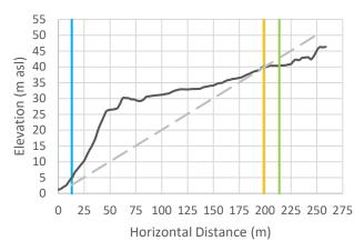
Cross-Section 17: Vertical exaggeration = 3. The black line is the cross-sectional data. The blue line is the Natural Boundary position with 1 m SLR, the orange line is the calculated setback, and the green line is the calculated setback plus 15 m.
