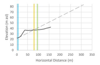
Cross-Section r-44: Vertical exaggeration = 2.5. The black line is the crosssectional data. The blue line is the toe of slope, the orange line is the calculated setback, and the green line is the calculated setback plus 15 m.
