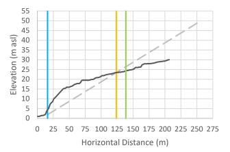
Cross-Section 4: Vertical exaggeration = 3. The black line is the cross-sectional data. The blue line is the Natural Boundary position with 1 m SLR, the orange line is the calculated setback, and the green line is the calculated setback plus 15 m.
