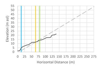
Cross-Section 51: Vertical exaggeration = 3. The black line is the cross-sectional data. The blue line is the Natural Boundary position with 1 m SLR, the orange line is the calculated setback, and the green line is the calculated setback plus 15 m.
