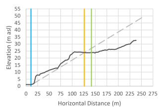
Cross-Section 15: Vertical exaggeration = 3. The black line is the cross-sectional data. The blue line is the Natural Boundary position with 1 m SLR, the orange line is the calculated setback, and the green line is the calculated setback plus 15 m.
