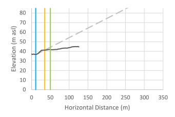
Cross-Section r-35: Vertical exaggeration = 2.5. The black line is the crosssectional data. The blue line is the toe of slope, the orange line is the calculated setback, and the green line is the calculated setback plus 15 m.
