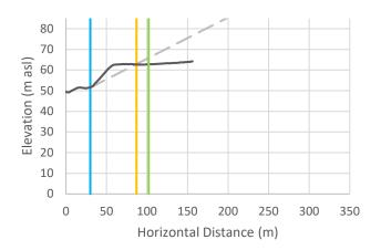
Cross-Section r-1555: Vertical exaggeration = 2.5. The black line is the crosssectional data. The blue line is the toe of slope, the orange line is the calculated setback, and the green line is the calculated setback plus 15 m.
