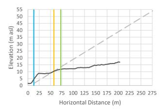
Cross-Section 49: Vertical exaggeration = 3. The black line is the cross-sectional data. The blue line is the Natural Boundary position with 1 m SLR, the orange line is the calculated setback, and the green line is the calculated setback plus 15 m.
