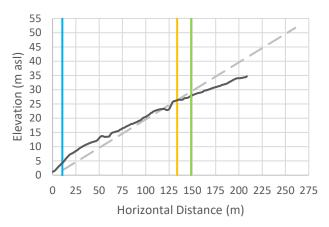
Cross-Section 11: Vertical exaggeration = 3. The black line is the cross-sectional data. The blue line is the Natural Boundary position with 1 m SLR, the orange line is the calculated setback, and the green line is the calculated setback plus 15 m.
