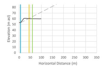
Cross-Section r-11: Vertical exaggeration = 2.5. The black line is the crosssectional data. The blue line is the toe of slope, the orange line is the calculated setback, and the green line is the calculated setback plus 15 m.
