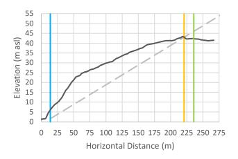
Cross-Section 37: Vertical exaggeration = 3. The black line is the cross-sectional data. The blue line is the Natural Boundary position with 1 m SLR, the orange line is the calculated setback, and the green line is the calculated setback plus 15 m.
