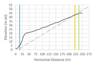
Cross-Section 35: Vertical exaggeration = 3. The black line is the cross-sectional data. The blue line is the Natural Boundary position with 1 m SLR, the orange line is the calculated setback, and the green line is the calculated setback plus 15 m.
