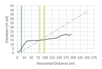
Cross-Section 13: Vertical exaggeration = 3. The black line is the cross-sectional data. The blue line is the Natural Boundary position with 1 m SLR, the orange line is the calculated setback, and the green line is the calculated setback plus 15 m.
