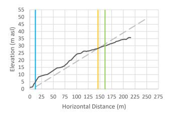
Cross-Section 8: Vertical exaggeration = 3. The black line is the cross-sectional data. The blue line is the Natural Boundary position with 1 m SLR, the orange line is the calculated setback, and the green line is the calculated setback plus 15 m.
