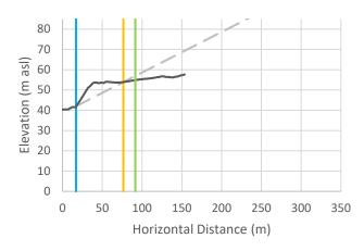
Cross-Section r-19: Vertical exaggeration = 2.5. The black line is the crosssectional data. The blue line is the toe of slope, the orange line is the calculated setback, and the green line is the calculated setback plus 15 m.
