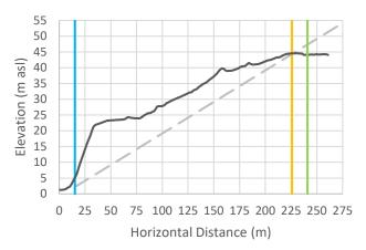
Cross-Section 36: Vertical exaggeration = 3. The black line is the cross-sectional data. The blue line is the Natural Boundary position with 1 m SLR, the orange line is the calculated setback, and the green line is the calculated setback plus 15 m.
