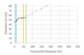
Cross-Section r-12: Vertical exaggeration = 2.5. The black line is the crosssectional data. The blue line is the toe of slope, the orange line is the calculated setback, and the green line is the calculated setback plus 15 m.
