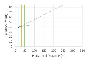
Cross-Section r-37: Vertical exaggeration = 2.5. The black line is the crosssectional data. The blue line is the toe of slope, the orange line is the calculated setback, and the green line is the calculated setback plus 15 m.
