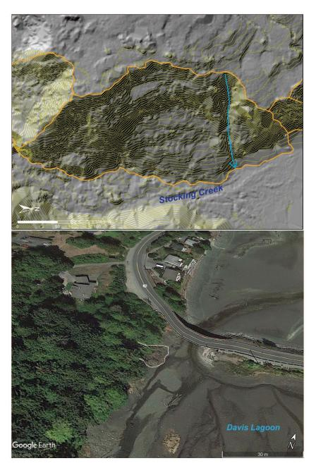
Figure 13. Landslide delineated in orange estimated to have been active within the last 500 years due to observed gully feature shown by blue arrow (above). Landslide estimated to have been active within the last 5 years due to observed deposit delineated in white in 2016 Google Earth imagery but not in available years of previous imagery (below).
