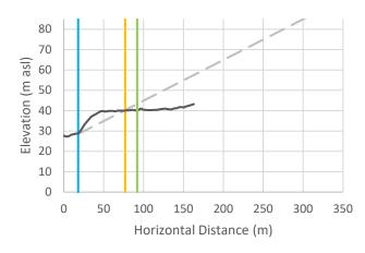
Cross-Section r-31: Vertical exaggeration = 2.5. The black line is the crosssectional data. The blue line is the toe of slope, the orange line is the calculated setback, and the green line is the calculated setback plus 15 m.
