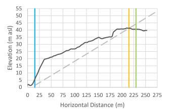
Cross-Section 34: Vertical exaggeration = 3. The black line is the cross-sectional data. The blue line is the Natural Boundary position with 1 m SLR, the orange line is the calculated setback, and the green line is the calculated setback plus 15 m.
