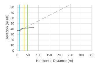
Cross-Section r-36: Vertical exaggeration = 2.5. The black line is the crosssectional data. The blue line is the toe of slope, the orange line is the calculated setback, and the green line is the calculated setback plus 15 m.
