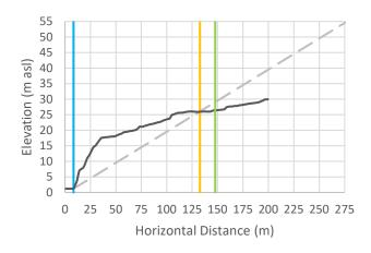
Cross-Section 32: Vertical exaggeration = 3. The black line is the cross-sectional data. The blue line is the Natural Boundary position with 1 m SLR, the orange line is the calculated setback, and the green line is the calculated setback plus 15 m.
