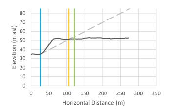
Cross-Section r-22: Vertical exaggeration = 2.5. The black line is the cross-sectional data. The blue line is the toe of slope, the orange line is the calculated setback, and the green line is the calculated setback plus 15 m.
