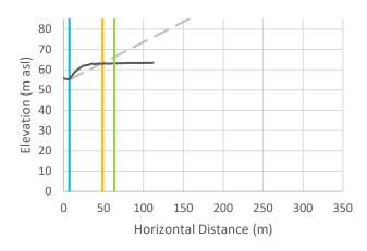
Cross-Section r-7: Vertical exaggeration = 2.5. The black line is the crosssectional data. The blue line is the toe of slope, the orange line is the calculated setback, and the green line is the calculated setback plus 15 m.
