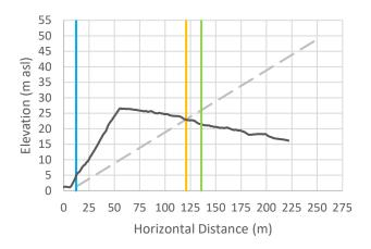
Cross-Section 25: Vertical exaggeration = 3. The black line is the cross-sectional data. The blue line is the Natural Boundary position with 1 m SLR, the orange line is the calculated setback, and the green line is the calculated setback plus 15 m.
