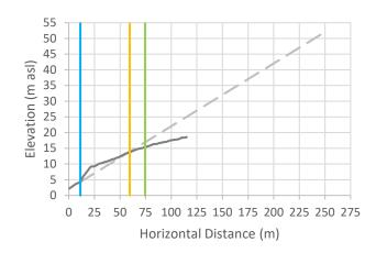
Cross-Section 2: Vertical exaggeration = 3. The black line is the cross-sectional data. The blue line is the Natural Boundary position with 1 m SLR, the orange line is the calculated setback, and the green line is the calculated setback plus 15 m.
