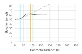
Cross-Section r-16: Vertical exaggeration = 2.5. The black line is the crosssectional data. The blue line is the toe of slope, the orange line is the calculated setback, and the green line is the calculated setback plus 15 m.
