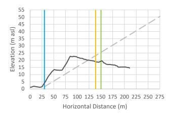
Cross-Section 26: Vertical exaggeration = 3. The black line is the cross-sectional data. The blue line is the Natural Boundary position with 1 m SLR, the orange line is the calculated setback, and the green line is the calculated setback plus 15 m.
