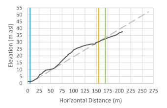
Cross-Section 10: Vertical exaggeration = 3. The black line is the cross-sectional data. The blue line is the Natural Boundary position with 1 m SLR, the orange line is the calculated setback, and the green line is the calculated setback plus 15 m.
