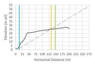
Cross-Section 41: Vertical exaggeration = 3. The black line is the cross-sectional data. The blue line is the Natural Boundary position with 1 m SLR, the orange line is the calculated setback, and the green line is the calculated setback plus 15 m.
