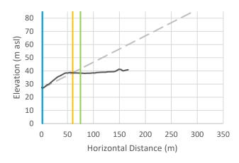
Cross-Section r-43: Vertical exaggeration = 2.5. The black line is the crosssectional data. The blue line is the toe of slope, the orange line is the calculated setback, and the green line is the calculated setback plus 15 m.
