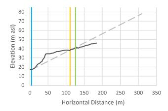
Cross-Section r-29: Vertical exaggeration = 2.5. The black line is the crosssectional data. The blue line is the toe of slope, the orange line is the calculated setback, and the green line is the calculated setback plus 15 m.
