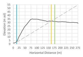
Cross-Section 24: Vertical exaggeration = 3. The black line is the cross-sectional data. The blue line is the Natural Boundary position with 1 m SLR, the orange line is the calculated setback, and the green line is the calculated setback plus 15 m.
