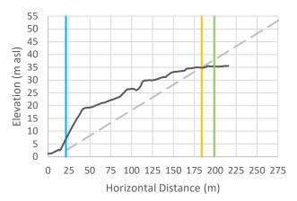
Cross-Section 33: Vertical exaggeration = 3. The black line is the cross-sectional data. The blue line is the Natural Boundary position with 1 m SLR, the orange line is the calculated setback, and the green line is the calculated setback plus 15 m.
