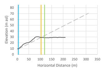
Cross-Section r-26: Vertical exaggeration = 2.5. The black line is the crosssectional data. The blue line is the toe of slope, the orange line is the calculated setback, and the green line is the calculated setback plus 15 m.
