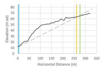
Cross-Section r-2: Vertical exaggeration = 2.5. The black line is the crosssectional data. The blue line is the toe of slope, the orange line is the calculated setback, and the green line is the calculated setback plus 15 m.
