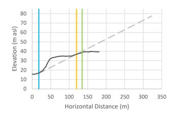
Cross-Section r-28: Vertical exaggeration = 2.5. The black line is the crosssectional data. The blue line is the toe of slope, the orange line is the calculated setback, and the green line is the calculated setback plus 15 m.
