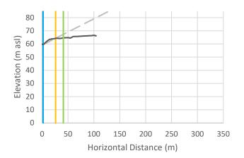
Cross-Section r-954: Vertical exaggeration = 2.5. The black line is the crosssectional data. The blue line is the toe of slope, the orange line is the calculated setback, and the green line is the calculated setback plus 15 m.
