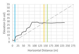
Cross-Section 40: Vertical exaggeration = 3. The black line is the cross-sectional data. The blue line is the Natural Boundary position with 1 m SLR, the orange line is the calculated setback, and the green line is the calculated setback plus 15 m.
