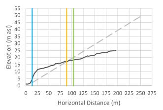
Cross-Section 3: Vertical exaggeration = 3. The black line is the cross-sectional data. The blue line is the Natural Boundary position with 1 m SLR, the orange line is the calculated setback, and the green line is the calculated setback plus 15 m.
