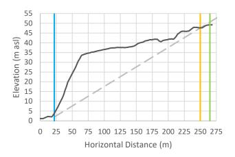
Cross-Section 19: Vertical exaggeration = 3. The black line is the cross-sectional data. The blue line is the Natural Boundary position with 1 m SLR, the orange line is the calculated setback, and the green line is the calculated setback plus 15 m.
