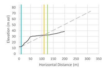
Cross-Section r-46: Vertical exaggeration = 2.5. The black line is the cross-sectional data. The blue line is the toe of slope, the orange line is the calculated setback, and the green line is the calculated setback plus 15 m.
