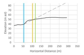
Cross-Section r-20: Vertical exaggeration = 2.5. The black line is the crosssectional data. The blue line is the toe of slope, the orange line is the calculated setback, and the green line is the calculated setback plus 15 m.
