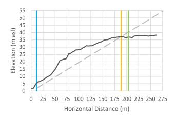
Cross-Section 38: Vertical exaggeration = 3. The black line is the cross-sectional data. The blue line is the Natural Boundary position with 1 m SLR, the orange line is the calculated setback, and the green line is the calculated setback plus 15 m.
