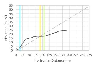
Cross-Section 47: Vertical exaggeration = 3. The black line is the cross-sectional data. The blue line is the Natural Boundary position with 1 m SLR, the orange line is the calculated setback, and the green line is the calculated setback plus 15 m.
