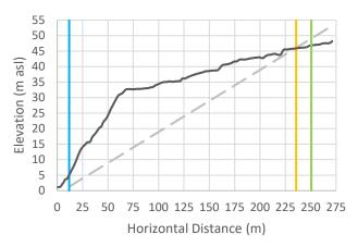
Cross-Section 18: Vertical exaggeration = 3. The black line is the cross-sectional data. The blue line is the Natural Boundary position with 1 m SLR, the orange line is the calculated setback, and the green line is the calculated setback plus 15 m.
