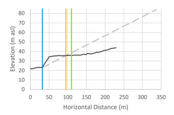
Cross-Section r-30: Vertical exaggeration = 2.5. The black line is the crosssectional data. The blue line is the toe of slope, the orange line is the calculated setback, and the green line is the calculated setback plus 15 m.
