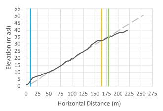
Cross-Section 9: Vertical exaggeration = 3. The black line is the cross-sectional data. The blue line is the Natural Boundary position with 1 m SLR, the orange line is the calculated setback, and the green line is the calculated setback plus 15 m.
