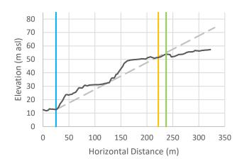
Cross-Section r-1: Vertical exaggeration = 2.5. The black line is the crosssectional data. The blue line is the toe of slope, the orange line is the calculated setback, and the green line is the calculated setback plus 15 m.
