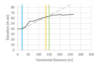
Cross-Section r-5: Vertical exaggeration = 2.5. The black line is the crosssectional data. The blue line is the toe of slope, the orange line is the calculated setback, and the green line is the calculated setback plus 15 m.
