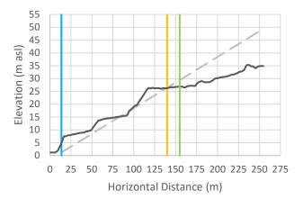
Cross-Section 16: Vertical exaggeration = 3. The black line is the cross-sectional data. The blue line is the Natural Boundary position with 1 m SLR, the orange line is the calculated setback, and the green line is the calculated setback plus 15 m.
