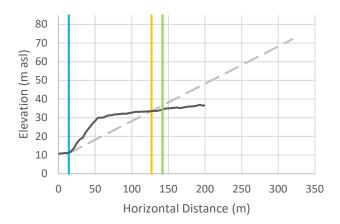
Cross-Section r-48: Vertical exaggeration = 2.5. The black line is the crosssectional data. The blue line is the toe of slope, the orange line is the calculated setback, and the green line is the calculated setback plus 15 m.
