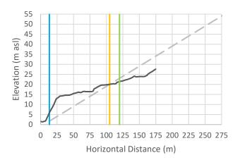
Cross-Section 52: Vertical exaggeration = 3. The black line is the cross-sectional data. The blue line is the Natural Boundary position with 1 m SLR, the orange line is the calculated setback, and the green line is the calculated setback plus 15 m.
