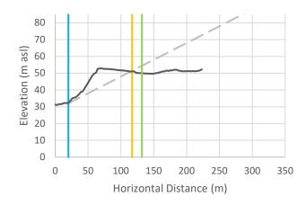
Cross-Section r-23: Vertical exaggeration = 2.5. The black line is the crosssectional data. The blue line is the toe of slope, the orange line is the calculated setback, and the green line is the calculated setback plus 15 m.
