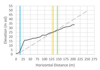
Cross-Section 5: Vertical exaggeration = 3. The black line is the cross-sectional data. The blue line is the Natural Boundary position with 1 m SLR, the orange line is the calculated setback, and the green line is the calculated setback plus 15 m.
