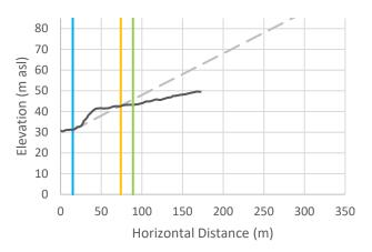
Cross-Section r-32: Vertical exaggeration = 2.5. The black line is the crosssectional data. The blue line is the toe of slope, the orange line is the calculated setback, and the green line is the calculated setback plus 15 m.
