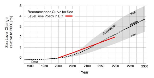
Figure 3. Recommended global sea level rise curve for planning and design in BC (Ausenco Sandwell, 2011).
