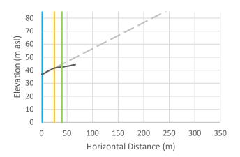
Cross-Section r-3959: Vertical exaggeration = 2.5. The black line is the crosssectional data. The blue line is the toe of slope, the orange line is the calculated setback, and the green line is the calculated setback plus 15 m.
