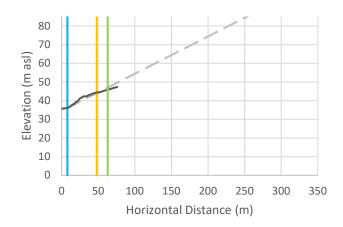
Cross-Section r-40: Vertical exaggeration = 2.5. The black line is the crosssectional data. The blue line is the toe of slope, the orange line is the calculated setback, and the green line is the calculated setback plus 15 m.
