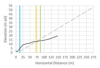
Cross-Section 27: Vertical exaggeration = 3. The black line is the cross-sectional data. The blue line is the Natural Boundary position with 1 m SLR, the orange line is the calculated setback, and the green line is the calculated setback plus 15 m.
