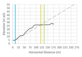
Cross-Section 42: Vertical exaggeration = 3. The black line is the cross-sectional data. The blue line is the Natural Boundary position with 1 m SLR, the orange line is the calculated setback, and the green line is the calculated setback plus 15 m.
