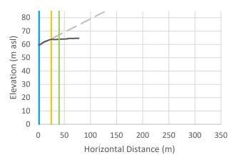
Cross-Section r-8: Vertical exaggeration = 2.5. The black line is the crosssectional data. The blue line is the toe of slope, the orange line is the calculated setback, and the green line is the calculated setback plus 15 m.
