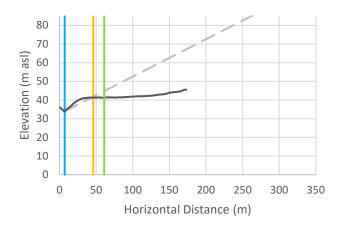
Cross-Section r-42: Vertical exaggeration = 2.5. The black line is the crosssectional data. The blue line is the toe of slope, the orange line is the calculated setback, and the green line is the calculated setback plus 15 m.
