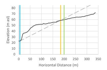
Cross-Section r-353: Vertical exaggeration = 2.5. The black line is the crosssectional data. The blue line is the toe of slope, the orange line is the calculated setback, and the green line is the calculated setback plus 15 m.
