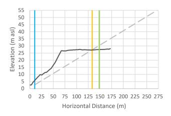
Cross-Section 44: Vertical exaggeration = 3. The black line is the cross-sectional data. The blue line is the Natural Boundary position with 1 m SLR, the orange line is the calculated setback, and the green line is the calculated setback plus 15 m.
