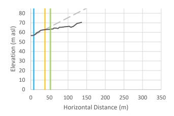
Cross-Section r-10: Vertical exaggeration = 2.5. The black line is the cross-sectional data. The blue line is the toe of slope, the orange line is the calculated setback, and the green line is the calculated setback plus 15 m.
