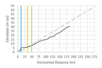
Cross-Section 50: Vertical exaggeration = 3. The black line is the cross-sectional data. The blue line is the Natural Boundary position with 1 m SLR, the orange line is the calculated setback, and the green line is the calculated setback plus 15 m.
