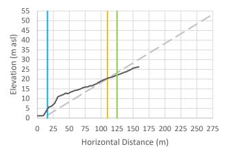
Cross-Section 28: Vertical exaggeration = 3. The black line is the cross-sectional data. The blue line is the Natural Boundary position with 1 m SLR, the orange line is the calculated setback, and the green line is the calculated setback plus 15 m.
