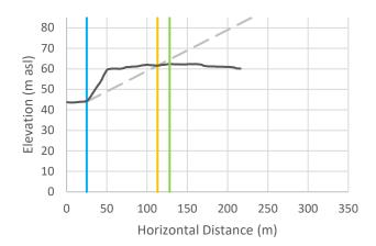
Cross-Section r-18: Vertical exaggeration = 2.5. The black line is the crosssectional data. The blue line is the toe of slope, the orange line is the calculated setback, and the green line is the calculated setback plus 15 m.
