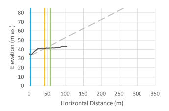
Cross-Section r-3358: Vertical exaggeration = 2.5. The black line is the crosssectional data. The blue line is the toe of slope, the orange line is the calculated setback, and the green line is the calculated setback plus 15 m.
