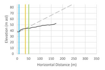
Cross-Section r-38: Vertical exaggeration = 2.5. The black line is the crosssectional data. The blue line is the toe of slope, the orange line is the calculated setback, and the green line is the calculated setback plus 15 m.
