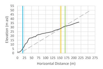
Cross-Section 7: Vertical exaggeration = 3. The black line is the cross-sectional data. The blue line is the Natural Boundary position with 1 m SLR, the orange line is the calculated setback, and the green line is the calculated setback plus 15 m.
