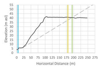
Cross-Section 22: Vertical exaggeration = 3. The black line is the cross-sectional data. The blue line is the Natural Boundary position with 1 m SLR, the orange line is the calculated setback, and the green line is the calculated setback plus 15 m.
