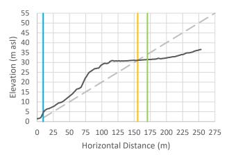
Cross-Section 39: Vertical exaggeration = 3. The black line is the cross-sectional data. The blue line is the Natural Boundary position with 1 m SLR, the orange line is the calculated setback, and the green line is the calculated setback plus 15 m.
