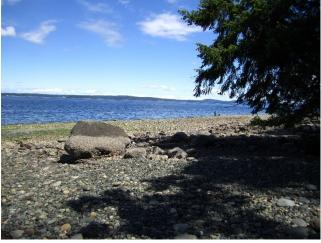
Photo 026: Looking SE over the beach. The upper beach face has 6-degree slope and  $\mathsf{D}_{50}$  of 30 mm.
