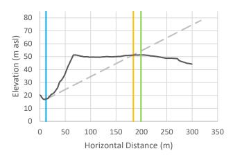
Cross-Section r-25: Vertical exaggeration = 2.5. The black line is the crosssectional data. The blue line is the toe of slope, the orange line is the calculated setback, and the green line is the calculated setback plus 15 m.
