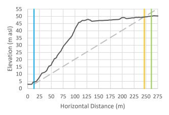
Cross-Section 21: Vertical exaggeration = 3. The black line is the cross-sectional data. The blue line is the Natural Boundary position with 1 m SLR, the orange line is the calculated setback, and the green line is the calculated setback plus 15 m.
