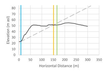
Cross-Section r-24: Vertical exaggeration = 2.5. The black line is the crosssectional data. The blue line is the toe of slope, the orange line is the calculated setback, and the green line is the calculated setback plus 15 m.
