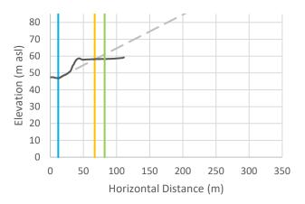
Cross-Section r-14: Vertical exaggeration = 2.5. The black line is the crosssectional data. The blue line is the toe of slope, the orange line is the calculated setback, and the green line is the calculated setback plus 15 m.
