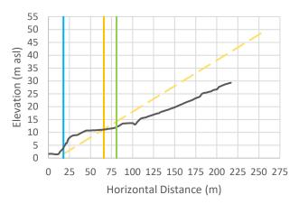
Cross-Section 12: Vertical exaggeration = 3. The black line is the cross-sectional data. The blue line is the Natural Boundary position with 1 m SLR, the orange line is the calculated setback, and the green line is the calculated setback plus 15 m.
