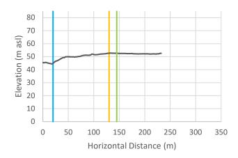
Cross-Section r-17: Vertical exaggeration = 2.5. The black line is the crosssectional data. The blue line is the toe of slope, the orange line is the calculated setback, and the green line is the calculated setback plus 15 m.
