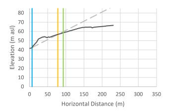
Cross-Section r-6: Vertical exaggeration = 2.5. The black line is the crosssectional data. The blue line is the toe of slope, the orange line is the calculated setback, and the green line is the calculated setback plus 15 m.
