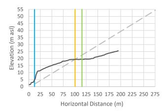
Cross-Section 46: Vertical exaggeration = 3. The black line is the cross-sectional data. The blue line is the Natural Boundary position with 1 m SLR, the orange line is the calculated setback, and the green line is the calculated setback plus 15 m.
