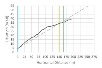
Cross-Section 43: Vertical exaggeration = 3. The black line is the cross-sectional data. The blue line is the Natural Boundary position with 1 m SLR, the orange line is the calculated setback, and the green line is the calculated setback plus 15 m.
