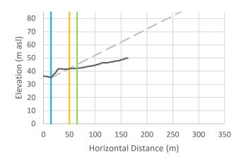
Cross-Section r-41: Vertical exaggeration = 2.5. The black line is the crosssectional data. The blue line is the toe of slope, the orange line is the calculated setback, and the green line is the calculated setback plus 15 m.
