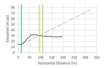
Cross-Section r-2757: Vertical exaggeration = 2.5. The black line is the crosssectional data. The blue line is the toe of slope, the orange line is the calculated setback, and the green line is the calculated setback plus 15 m.
