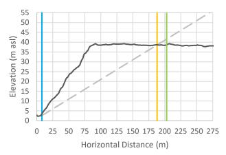
Cross-Section 23: Vertical exaggeration = 3. The black line is the cross-sectional data. The blue line is the Natural Boundary position with 1 m SLR, the orange line is the calculated setback, and the green line is the calculated setback plus 15 m.
