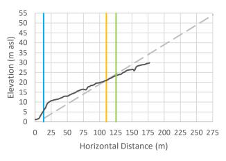
Cross-Section 31: Vertical exaggeration = 3. The black line is the cross-sectional data. The blue line is the Natural Boundary position with 1 m SLR, the orange line is the calculated setback, and the green line is the calculated setback plus 15 m.
