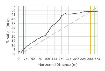
Cross-Section 20: Vertical exaggeration = 3. The black line is the cross-sectional data. The blue line is the Natural Boundary position with 1 m SLR, the orange line is the calculated setback, and the green line is the calculated setback plus 15 m.
