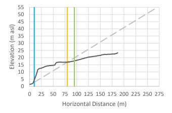
Cross-Section 48: Vertical exaggeration = 3. The black line is the cross-sectional data. The blue line is the Natural Boundary position with 1 m SLR, the orange line is the calculated setback, and the green line is the calculated setback plus 15 m.
