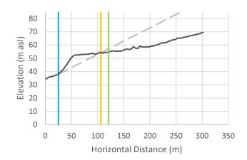
Cross-Section r-4: Vertical exaggeration = 2.5. The black line is the crosssectional data. The blue line is the toe of slope, the orange line is the calculated setback, and the green line is the calculated setback plus 15 m.
