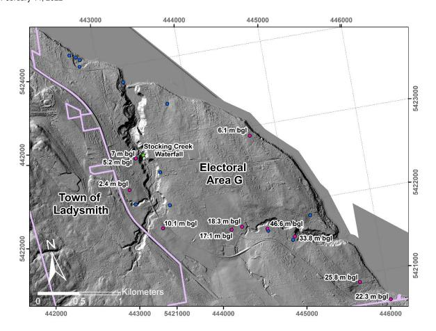
Figure 11. Water wells adjacent to the study area (FrontCounterBC, 2021). Water wells are shown in blue if no bedrock was encountered and shown in pink if bedrock was encountered. Water wells with record of bedrock are labeled with associated depth to bedrock in metres below ground level (m bgl). The location of Stocking Creek waterfall is also shown.
