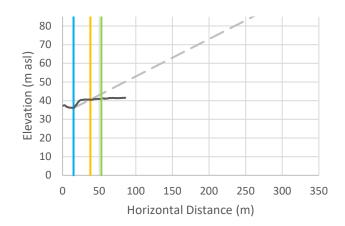
Cross-Section r-34: Vertical exaggeration = 2.5. The black line is the crosssectional data. The blue line is the toe of slope, the orange line is the calculated setback, and the green line is the calculated setback plus 15 m.
