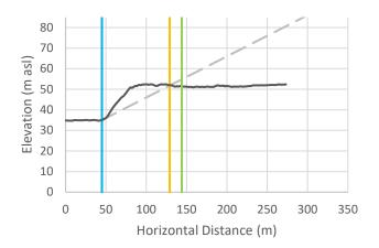
Cross-Section r-2156: Vertical exaggeration = 2.5. The black line is the crosssectional data. The blue line is the toe of slope, the orange line is the calculated setback, and the green line is the calculated setback plus 15 m.
