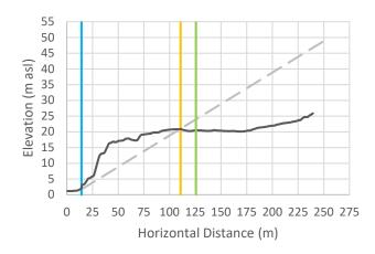
Cross-Section 14: Vertical exaggeration = 3. The black line is the cross-sectional data. The blue line is the Natural Boundary position with 1 m SLR, the orange line is the calculated setback, and the green line is the calculated setback plus 15 m.
