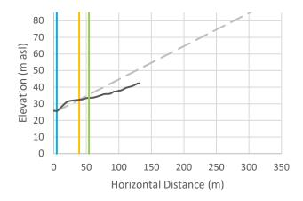
Cross-Section r-47: Vertical exaggeration = 2.5. The black line is the crosssectional data. The blue line is the toe of slope, the orange line is the calculated setback, and the green line is the calculated setback plus 15 m.
