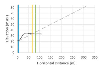
Cross-Section r-4560: Vertical exaggeration = 2.5. The black line is the crosssectional data. The blue line is the toe of slope, the orange line is the calculated setback, and the green line is the calculated setback plus 15 m.
