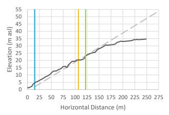
Cross-Section 30: Vertical exaggeration = 3. The black line is the cross-sectional data. The blue line is the Natural Boundary position with 1 m SLR, the orange line is the calculated setback, and the green line is the calculated setback plus 15 m.
