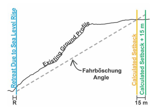
Figure 4. Diagram showing components contributing to recommended coastal slope stability setbacks.
