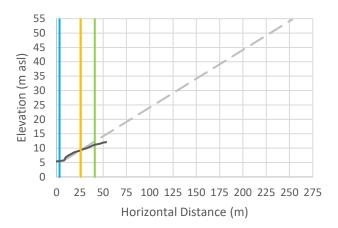
Cross-Section 1: Vertical exaggeration = 3. The black line is the cross-sectional data. The blue line is the Natural Boundary position with 1 m SLR, the orange line is the calculated setback, and the green line is the calculated setback plus 15 m.
