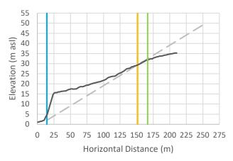
Cross-Section 6: Vertical exaggeration = 3. The black line is the cross-sectional data. The blue line is the Natural Boundary position with 1 m SLR, the orange line is the calculated setback, and the green line is the calculated setback plus 15 m.
