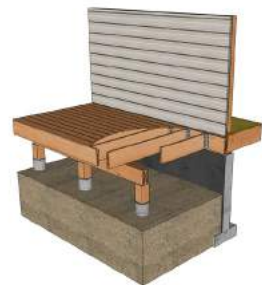
..... Open Deck - Ledger Attachment .....
