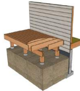
..... Open Deck - Independent Structure (Post Support) .....
