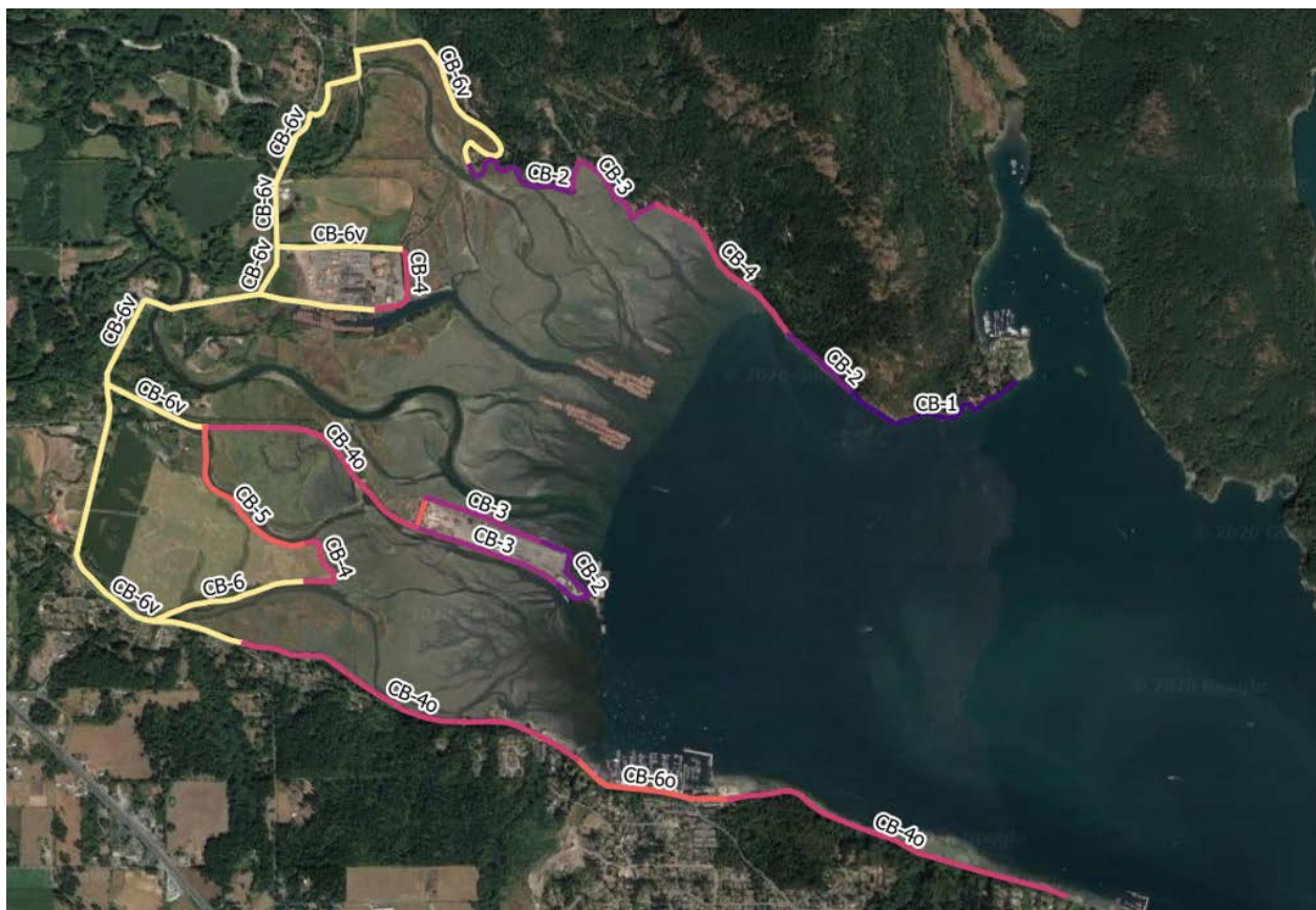
Figure 9-6: Shoreline reaches and wave effects for Cowichan Bay. Shoreline reach labels are differentiated by their wave run-up specific shoreline characteristics – no abbreviation for rip rap, ‘v’ for vegetation and ‘o’ for oblique
