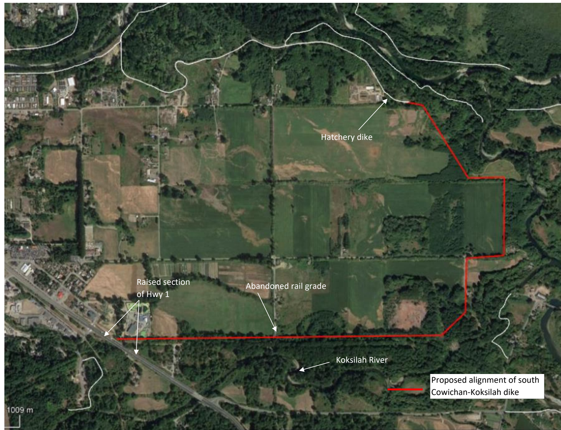
Figure 8-8: Proposed alignment of the south Cowichan-Koksilah dike.
