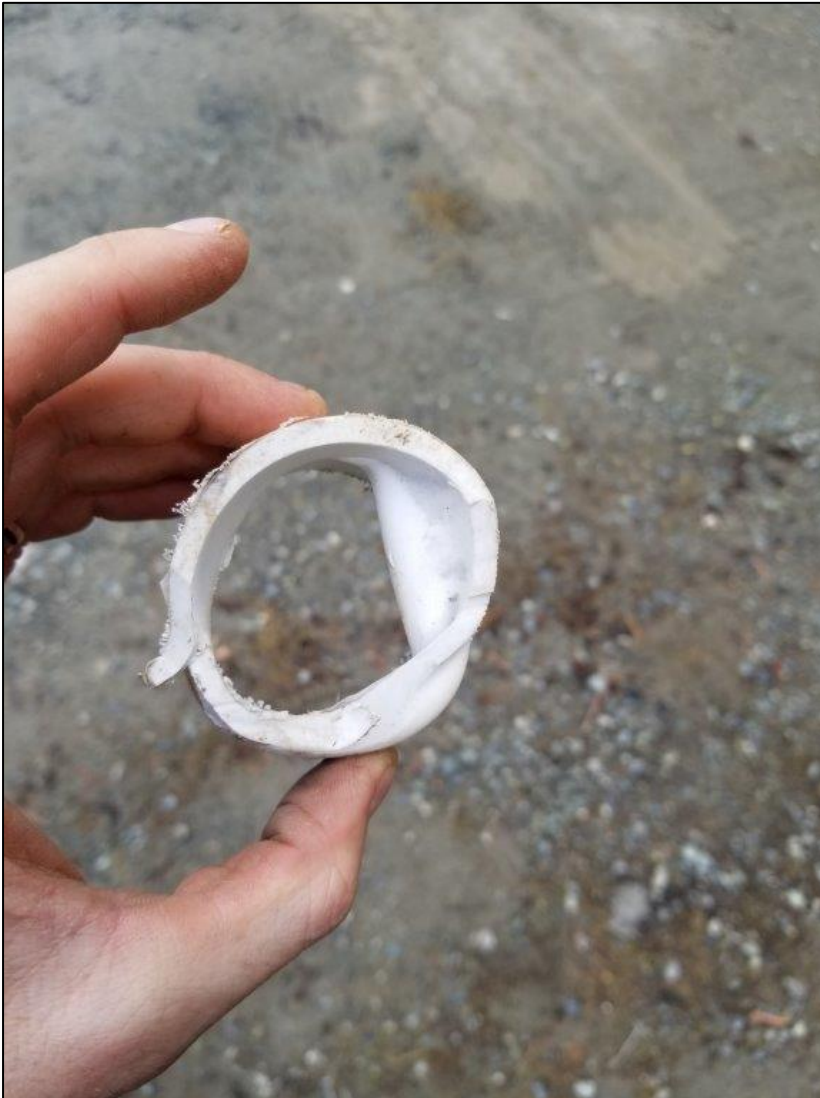
Photograph B5 (LEFT): Section of damaged PVC casing removed from MW12-3.
