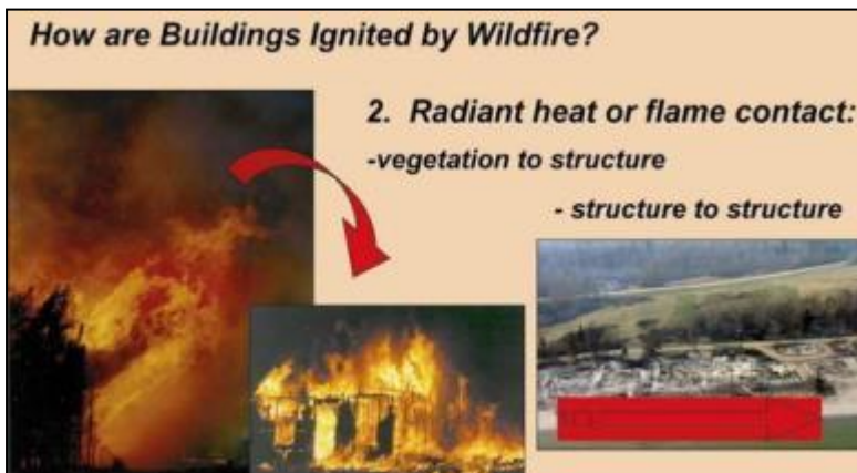
Figure 9. Radiant heat and flame contact allows fire to spread from vegetation to structure or from structure to structure.
